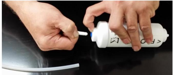
Step 3: Push your ¼” tubing into the quick connect fitting, until the tubing bottoms out. A clean, flat, and perpendicular cut works best.
