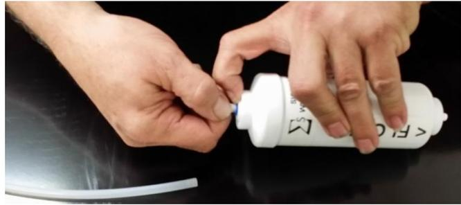
Step 2: Remove plug with a sharp pull.
